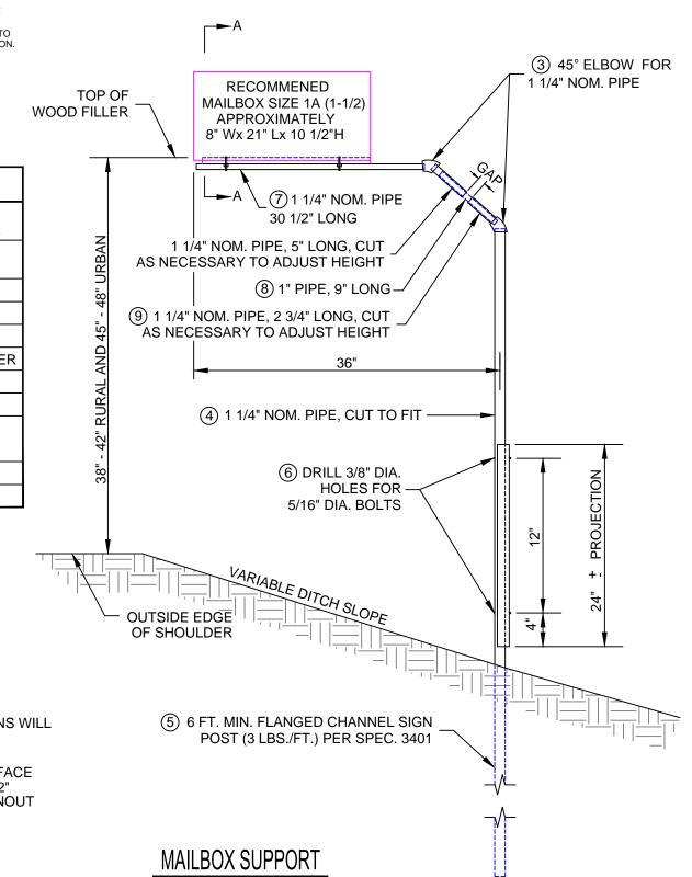
STEEL PIPE WITH FITTINGS AND STEEL POST
